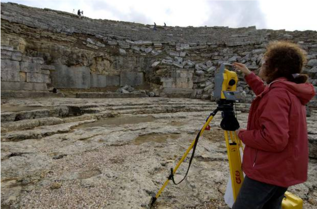
Cyrene, the Theatre-Amphitheatre during the works of 2006: application of the scanner laser per the survey three-dimensional of the cavea
