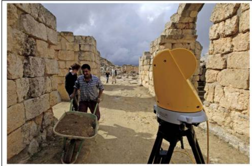
Cyrene, Theatre-Amphitheatre during the works of 2006: application of the laser scanner for the three-dimensional survey of the East Entrance
