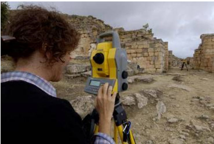
Cyrene, Theatre-Amphitheatre during the works of 2006: application of the scanner laser for the three-dimensional survey of the monument
